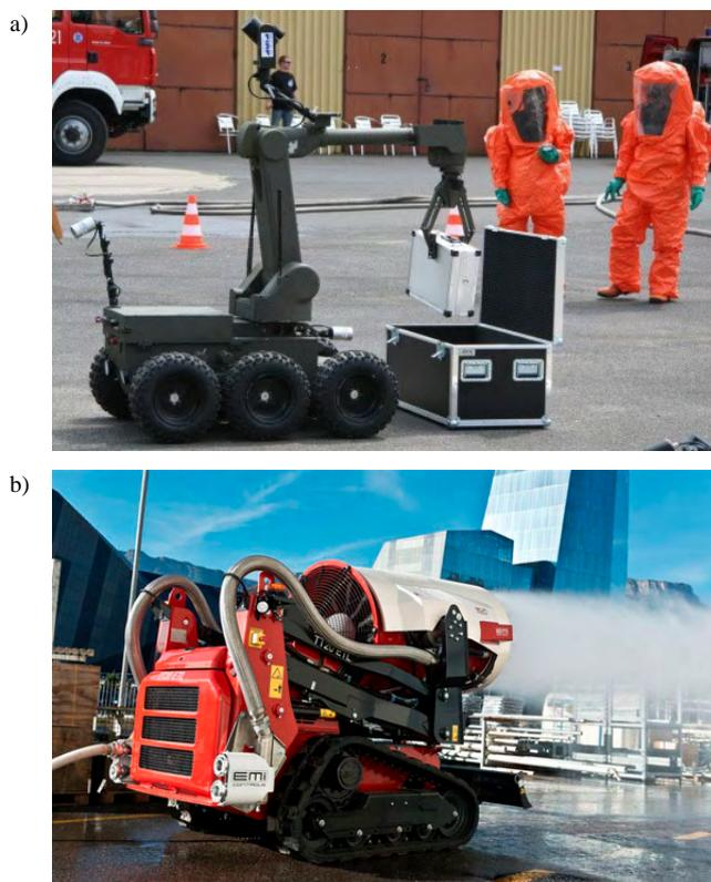
Fig. 1. Example of use UGV vehicles: a) operating in contaminated area [14], b) firefighting unmanned system [15]
