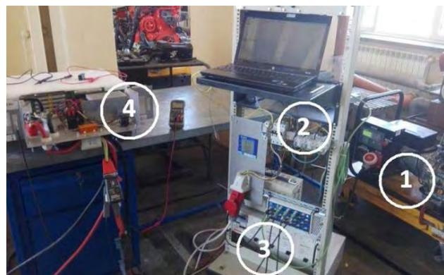
Fig. 4 Charging test stand: 1 – power generator, 2 – current-voltage parameters acquisition system, 3 – constant-current power station, 4 – battery
