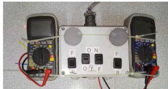
Fig. 8. Connected voltmeters for speed verification
