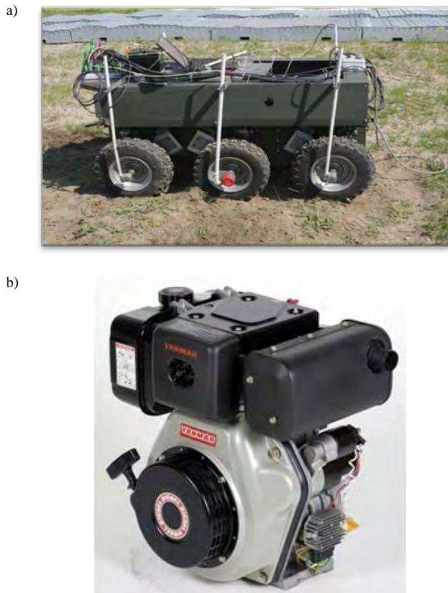
Fig. 2. a) investigated UGV with power transmission during tests, b) Diesel engine for vehicle's power generator [16]
