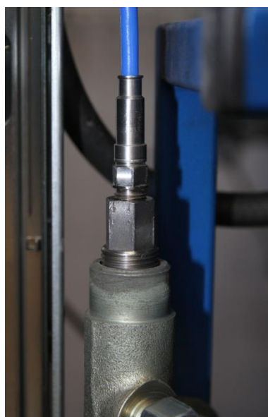
Fig. 1. STPiW-2 testing table: a) general view, b) AVL SL31D2000 pressure sensor fitted in the adapter: 1 – fuel injector tester, 2 – high-pressure pump tester, 3 – testing table control module, 4 – injectors, 5 – fuel dose measurements cylinders, 6 – high-pressure pump, 7 – overflow measurement cylinders
