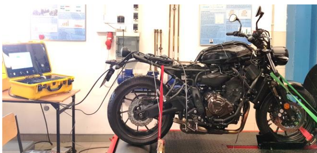
Fig. 5. Picture of the tested motorcycle along with the measuring apparatus on the designated dynamometer
