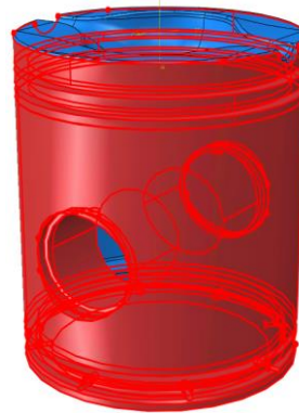
Fig. 6. The boundary condition of the piston's thermal load – side surfaces – temperature: 393 K, heat transfer coefficient: 500 W/(m 2 K)
