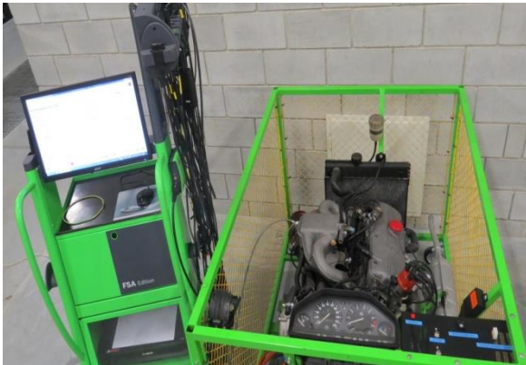
Fig. 1. Test stand with BMW M10B18 engine
