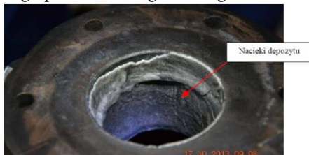
Fig. 13. Internal wall after the tests with cooled exhaust pipe (entry to the pipe) [0]
