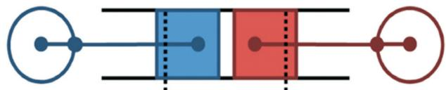
Fig. 1. Schematic of opposed piston two-stroke engine
