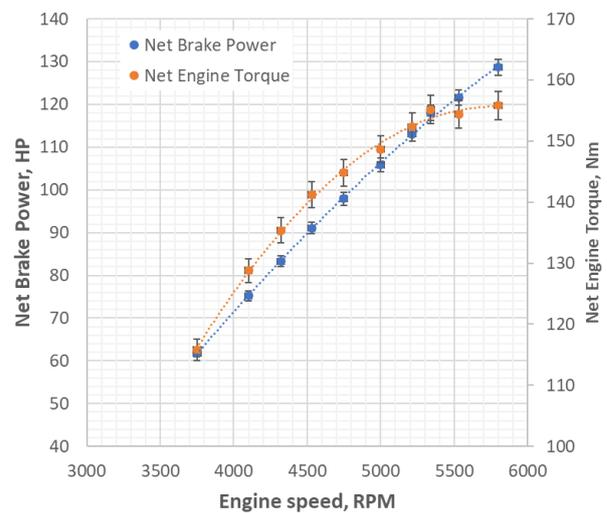
Fig. 2. Performance characteristics of the engine [26]
