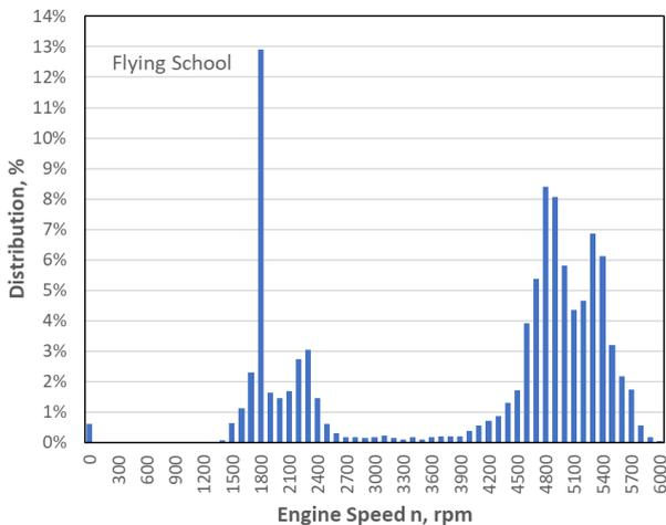
Fig. 6. Distribution of engine speed during training flights
