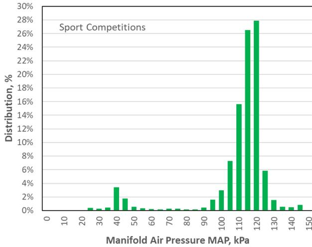
Fig. 9. Distribution of manifold air pressure during the sport competition
