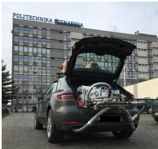
Fig. 1. The tested vehicle with PEMS apparatus
