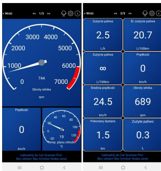
Fig. 5. Example of real-time preview of engine operating parameters using the "Car Scanner" application
