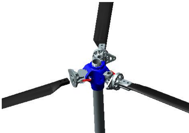
Fig. 6. Visualisation of the MBD main rotor base model
