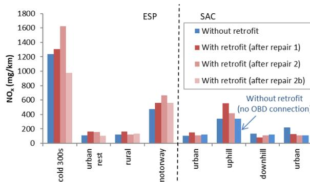
Fig. 7. NO<sub>x</sub> results for the on-road tests
