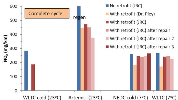
Fig. 6. NO<sub>x</sub> results for the complete cycles. "Regen" means that regeneration took place
