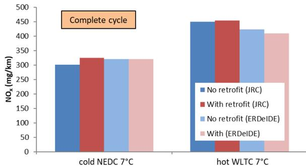
Fig. 3. NO<sub>x</sub> results for the complete cycles
