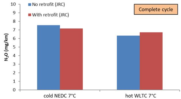
Fig. 5. N<sub>2</sub>O results for the complete cycles
