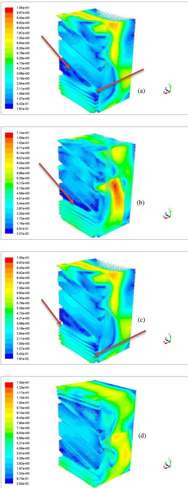
Fig.11. Velocity vector fields [m/s] (a) without guide vanes, (b) with one stream guide vane, (c) with two stream guide vanes, (d) with stream separation. The dead-zones and adverse flow events are indicated by red arrows
