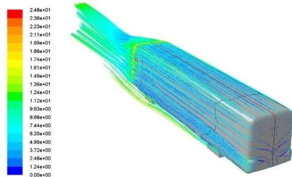
Fig. 6. Streamlines based on velocity [m/s] – view of the bus from the front of the vehicle on the side of radiator mounting
