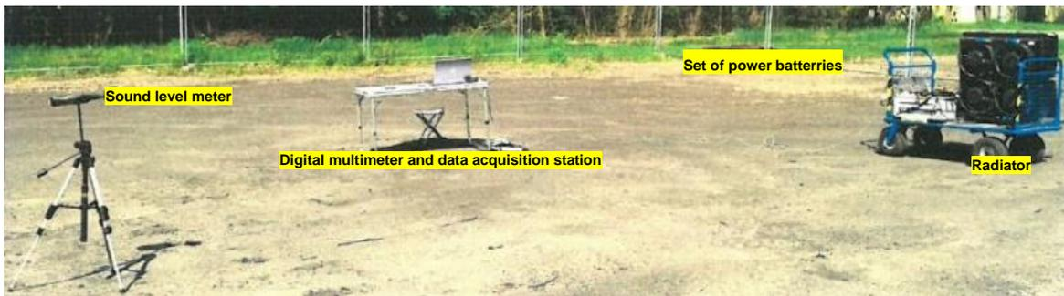
Fig. 14. The view of the test stand during the performance of acoustic pressure tests of the radiator in the field conditions at the Military Institute of Armoured and Automotive Technology (test certificate 41/LPE/2020)
