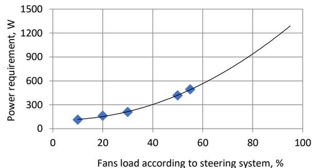
Fig. 16. Cooling fan power consumption depending on the % of the load defined by the control system in laboratory conditions
