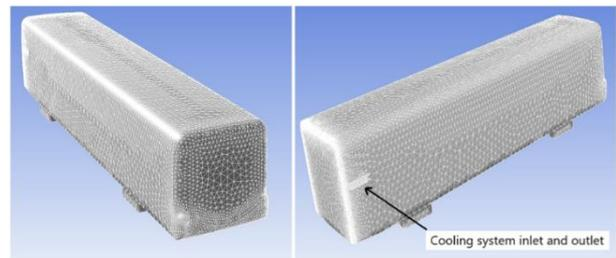
Fig. 5. A discrete model of an electric vehicle (bus)
