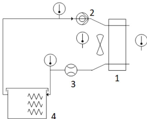
Fig. 4. A schematic diagram of the test stand: 1 – radiator, 2 – pump, 3 – flow meter, 4 – buffer tank
