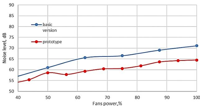
Fig. 15. Results of noise level measurements – comparison of the base and prototype versions (developed on the basis of numerical analysis)
