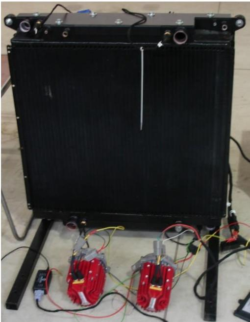
Fig. 1. The research object – radiator with an air distribution system, equipped with a set of fans, liquid and air temperature sensors, a wire harness adapted to communication via the CAN 2.0B bus, with a transmission speed of 250 Kbps
