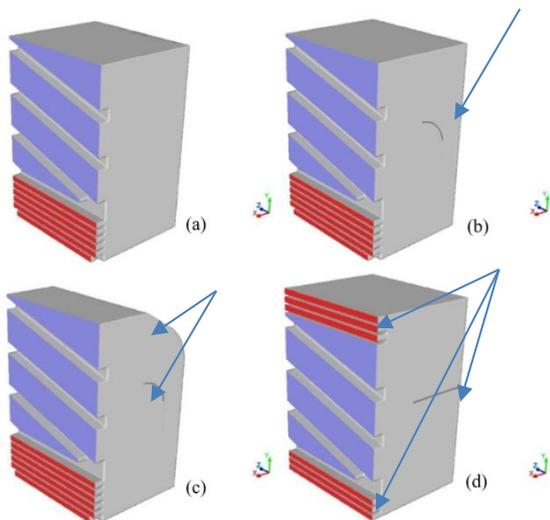
Fig. 9. Geometric models: (a) without guide vanes, (b) with one stream guide vane, (c) with two stream guide vanes, (d) with stream separation. The changes in geometry are indicated by arrows
