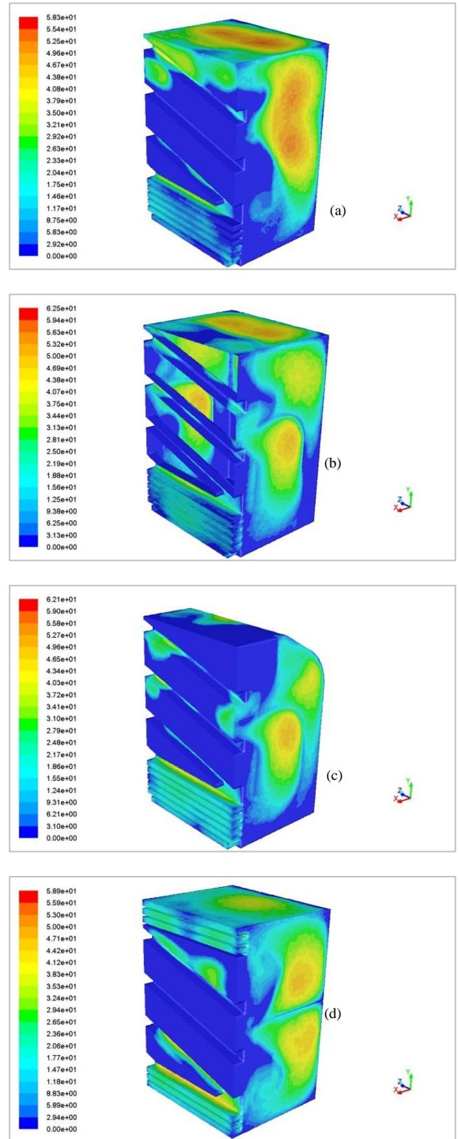
Fig. 10. Acoustic pressure fields [dB]: (a) without guide vanes, (b) with one stream guide vane, (c) with two stream guide vanes, (d) with stream separation
