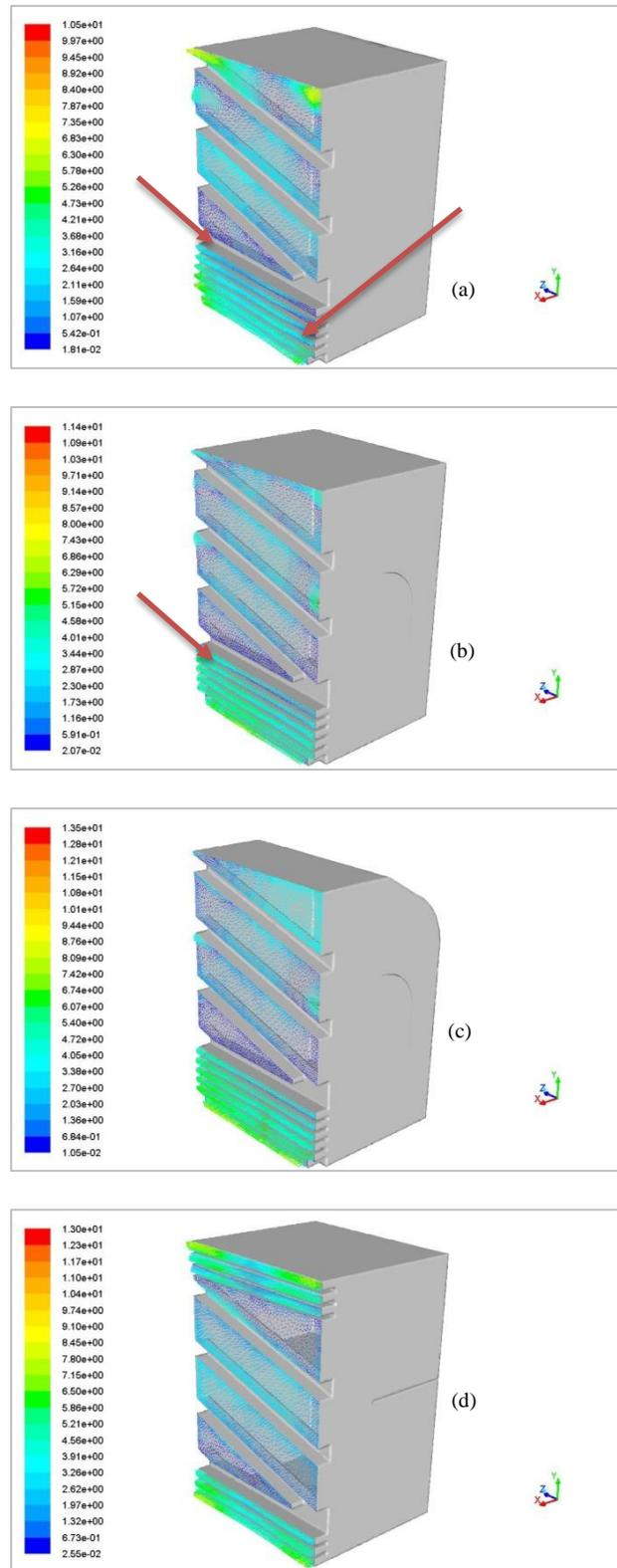
Fig. 12. Inlet and outlet velocity vector fields [m/s] (a) without guide vanes, (b) with one stream guide vane, (c) with two stream guide vanes, (d) with stream separation. The dead-zones and adverse flow events are indicated by red arrows
