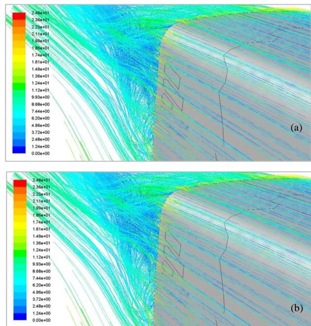
Fig. 7. Streamlines based on velocity [m/s] – radiator inlet grilles and streamlines with operating fans: view of the inlet grilles: a) when the vehicle is moving without the cooling system on, b) when the vehicle is moving with the cooling system on
