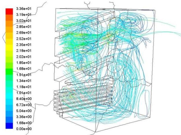
Fig. 8. Streamlines based on velocity [m/s] inside the radiator box
