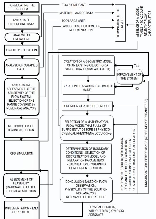
Fig. 2. Scheme of Zawiślak's method 'Design and modernisation of machines and flow systems using CFD software' [13]
