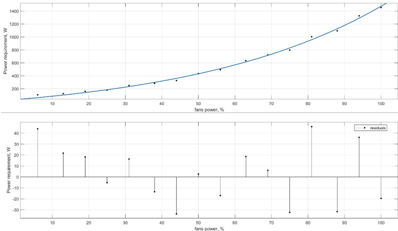
Fig. 17. Observed parameters of power requirement, W, with respect to fan load, %, in field conditions
