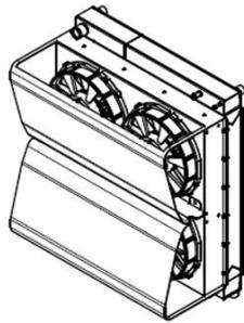
Fig. 13. Selected radiator geometry
