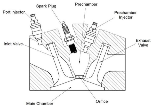
Fig. 7. Simplified scheme of hydrogen combustion prechamber system
