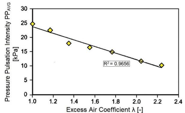
Fig. 3. Excess air influence on pressure pulsation intensity [25]
