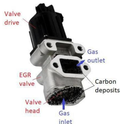
Fig. 1. EGR-valve covered with Carbon Deposits (CDs)
