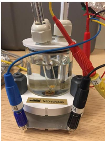
Fig. 1. The measurement site for corrosion tests
