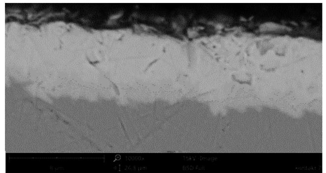
Fig. 6. Scanning microscope image of sample number 4 – a continuous layer with even coating thickness, visible impurities in the coating
