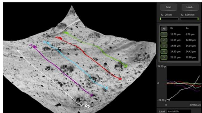
Fig. 13. Sample number 3, measurement 2 – 3D view of the test surface
