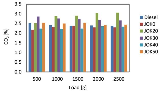
Fig. 9. Variation of CO<sub>2</sub> for JOK blends with increase in load
