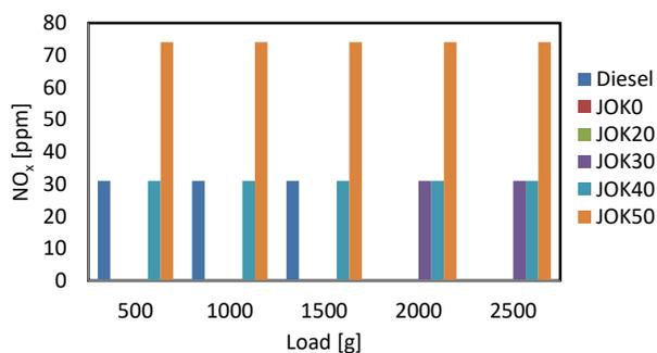
Fig. 11. Variation of NO<sub>x</sub> for JOK blends with increase in load
