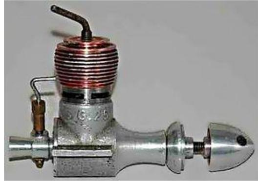
Fig. 3. Polish self-ignition engine “Jaskółka” with a capacity of  $2.5 \text{ cm}^3$  [26]
