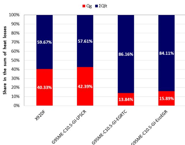
Fig. 3. Share of exhaust gas and low-temperature waste heat in the sum of heat losses
