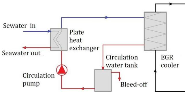
Fig. 1. Overview of the EGR cooling system [21]
