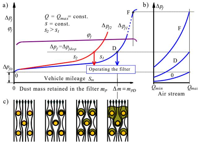
Fig. 1. The essence of baffle filters: a) filtration efficiency  $\varphi$  and pressure drop  $\Delta p_f$  of the air filter with filter media during use (1 – low dust concentration, 2 – high dust concentration), b) aerodynamic characteristics  $\Delta p_f = f(Q)$  of the air filter, c) changes in the absorptive capacity of the filter bed when loaded with dust
