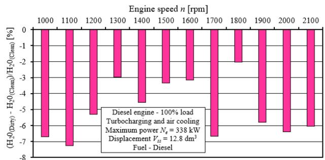
Fig. 27. Relative change in  $H_2O$  emissions from the engine for each speed  $n$  caused by a change in the condition of the „Dirty” air filter, relative to power with the air filter in „Clean” condition
