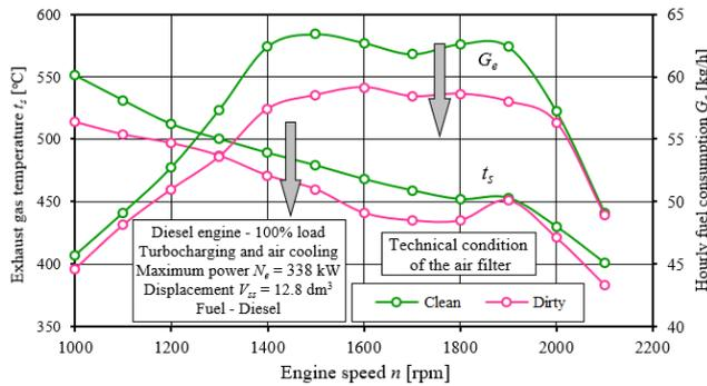
Fig. 10. The effect of technical conditions of the air filter on changes in hourly fuel consumption  $G_e$  and exhaust gas temperature  $t_s$  at the exit of the turbocharger of the engine under study as a function of engine speed  $n$
