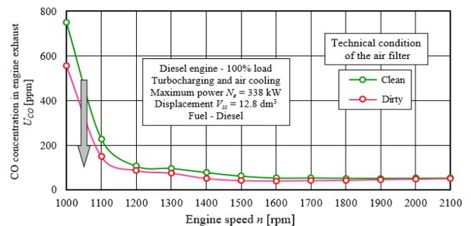
Fig. 15. CO concentration in the exhaust gas of the tested engine caused by a change in the condition of the air filter: "Clean" "Dirty"
