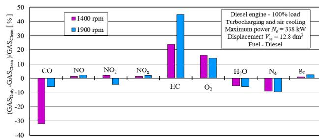
Fig. 28. Relative change in power  $N_e$  and specific fuel consumption  $g_e$  and emissions from the VOLVO DC13C460 engine for two characteristic speeds  $n = 1400$  rpm and  $n = 1900$  rpm caused by a change in the technical condition of the "Dirty" air filter, relative to power  $N_e$  and  $g_e$  emissions with the air filter in the "Clean" condition
