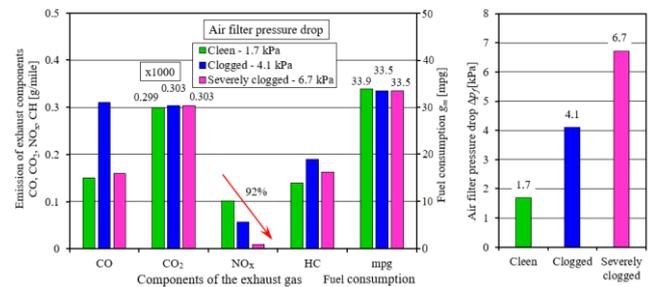
Fig. 2. The effect of an increase in baffled air filter flow resistance on emissions of exhaust components: CO,  $\text{CO}_2$ ,  $\text{NO}_x$  and fuel consumption of the engine of a Dodge Ram 2500 Truck 6.7 L. Figure made by the authors based on data from the paper [62]
