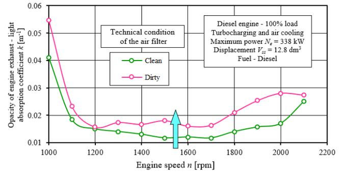
Fig. 11. Exhaust gas opacity of the VOVLO DC13C460 engine – light absorption coefficient  $k$  (absorption) as a function of engine speed  $n$  for two technical states of the air filter: „Clean” and „Dirty”.
