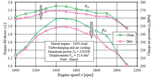
Fig. 6. Change in engine fill factor  $\eta_v$  and charge air pressure  $p_d$  in the intake manifold of the VOVLO DC13C460 engine depending on engine speed  $n$  caused by two technical states of the air filter: "Clean", "Dirty"
