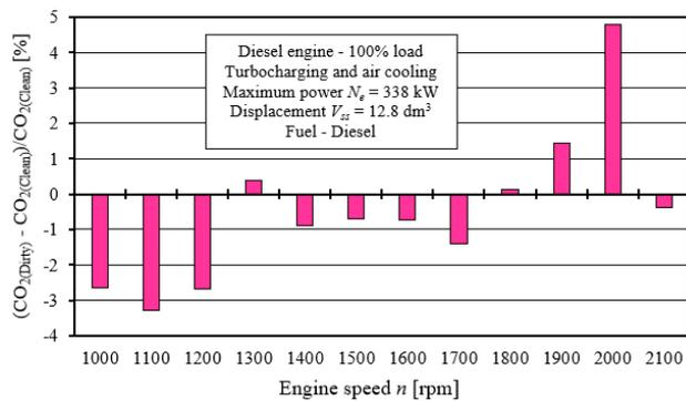
Fig. 14. Relative change in CO<sub>2</sub> emissions from the engine for different speeds due to a change in the condition of the air filter, relative to power with the air filter in „Clean” condition
