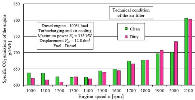
Fig. 13. Unit CO<sub>2</sub> emissions from the engine due to a change in the condition of the air filter "Clean"–"Dirty"
