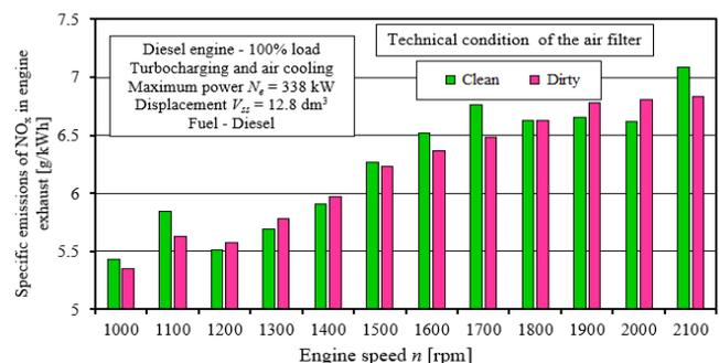
Fig. 19. Unit emission of  $\text{NO}_x$  in engine exhaust due to change in condition of air filter "Clean"–"Dirty"
