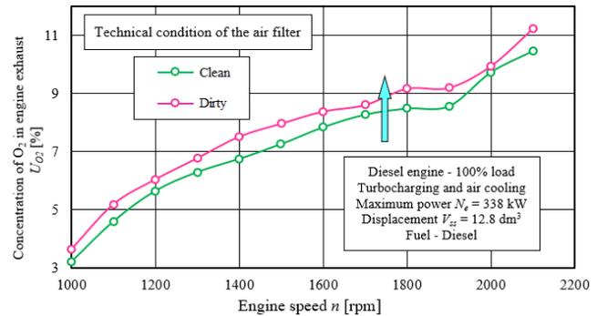
Fig. 22.  $\text{O}_2$  concentration in the engine exhaust caused by a change in the condition of the air filter: "Clean"–"Dirty"
