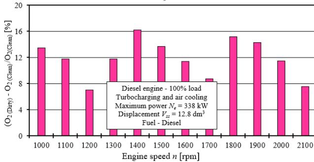
Fig. 24. Relative change in  $O_2$  emission from the engine for particular rotational speeds  $n$  caused by a change in the technical condition of the air filter, in relation to the power with the air filter in the „Clean” technical condition
