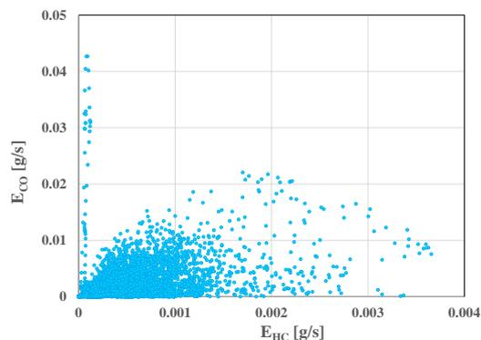
Fig. 14. Correlation relationship between the carbon monoxide emission intensity – E<sub>CO</sub> and the hydrocarbon emission intensity – E<sub>HC</sub> during the RDE test
