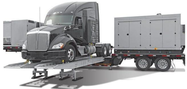
Fig. 2. Render of the mobile chassis dynamometer solution by Taylor Dyno [19]
