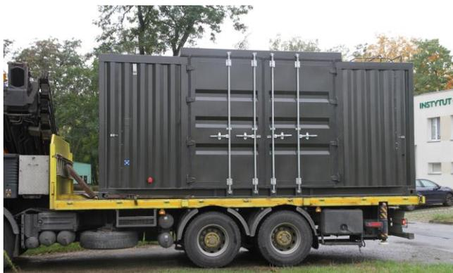
Fig. 8. The diag- dyno station transported on a truck chassis
