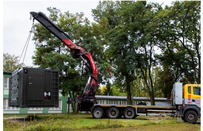
Fig. 9. The diag- dyno station during unloading using a hydraulic truck crane
