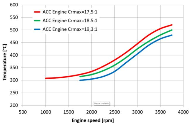
Fig. 8. Exhaust gas temperature measured in the ACC engine as a function of engine speed for maximum engine torque and various compression ratios
