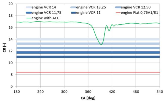
Fig. 2. CR changes in an engine with ACC within a portion of a single working cycle against the background of constant CR values in old and new SI engines and fixed CR values actuated by the control system in an engine with a VCR system
