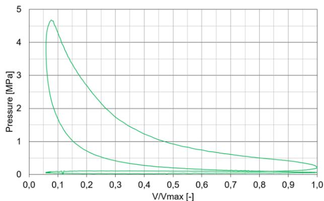
Fig. 11. Indicated pressure in the ACC engine under  $CR_{max} = 17.5: 1$  at engine speed of 3750 rpm
