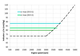
Fig. 4. The effect of the indicator  $\gamma_{\rm fm}$  on the achieved maximum ACC engine speed
