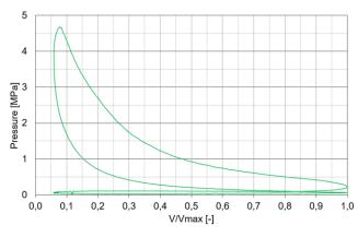
Fig. 11. Indicated pressure in the ACC engine under  $CR_{max} = 17.5$ : 1 at engine speed of 3750 rpm
