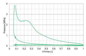
Fig. 9. Indicated pressure in the ACC engine under  $CR_{max} = 17.5$ : 1 at engine speed of 1000 rpm
