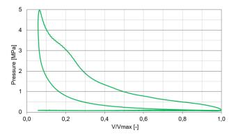
Fig. 10. Indicated pressure in the ACC engine under  $CR_{max} = 17.5$ : 1 at engine speed of 1900 rpm
