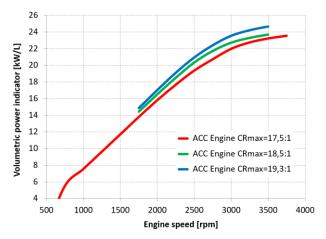
Fig. 6. Power for the maximum torque of the ACC engine with a displacement of one liter obtained for three CR<sub>max</sub> values
