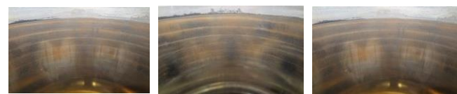
Fig. 8. Photograph of the surface of cylinders no. 3, 5 and 8 after the engine verification test
