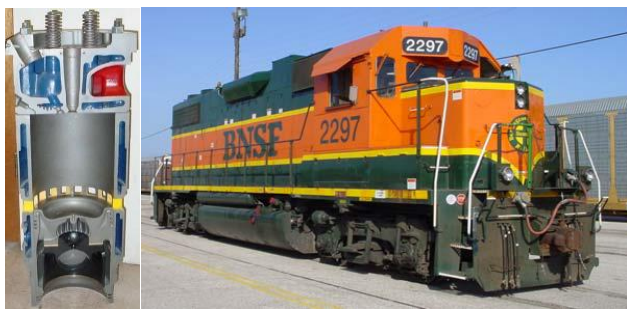
Fig. 1. EMD 645-E power assembly and GP38-2 locomotive [6]
