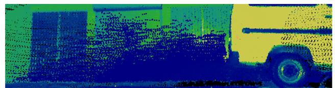
Fig. 2. A section of the point cloud generated by the lidar during the investigation of the water splash by the wheel
