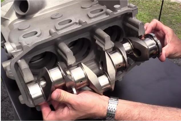
Fig. 2. View of the Gemini 100 engine crankshaft [1]
