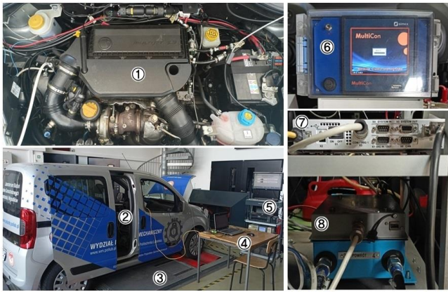
Fig. 1. Test bench: 1 – 1.3 Multijet engine, 2 – Fiat Qubo, 3 – Dynorace DF4FS-HLS chassis dynamometer, 4 – computer with software: AVL Indicom, MultiEcuScan and dedicated gas control software, 5 – MAHA MET 6.3 exhaust gas analyzer, 6 – MultiCon CMC-99 data logger, 7 – AVL IndiMicro 602 measuring system, 8 – ZPR 1-B/S fuel consumption meter
