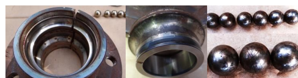
Fig. 9. Outer and inner rings of the left rear wheel bearing with visible surface fatigue and pitting damage on the raceways
