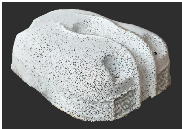
Fig. 9. The result of aggregating data using the iPhone TrueDepth for the spray-coated part
