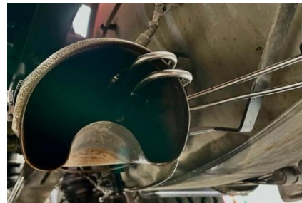
Fig. 3. a) Axion R/S+PM portable emission measurement system, b) PEMS probes installed on the truck's exhaust system.
