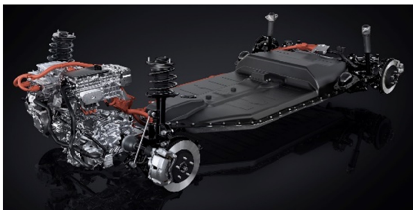
Fig. 13. Arrangement of the components of the electric driveline (Lexus UX) [8]
