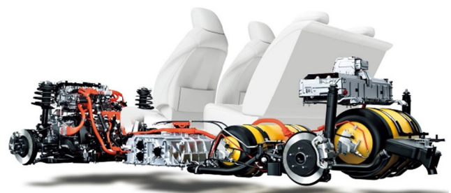
Fig. 14. Arrangement of the components of the fuel cell driveline (Toyota Mirai) [8]
