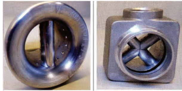
Fig. 20. The examples of throat constructions from gas mixers for different engines (reproduced from [10])
