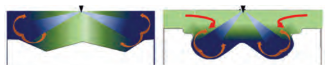
Fig. 18. Piston bowl geometries and injection configurations in a different fuel supply systems in RCCI engines (reproduced from Applied Energy [19] with permission from Elsevier)
