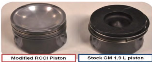
Fig. 14. Photo of modified RCCI piston and stock GM 1.9 L piston (reproduced from [1])
