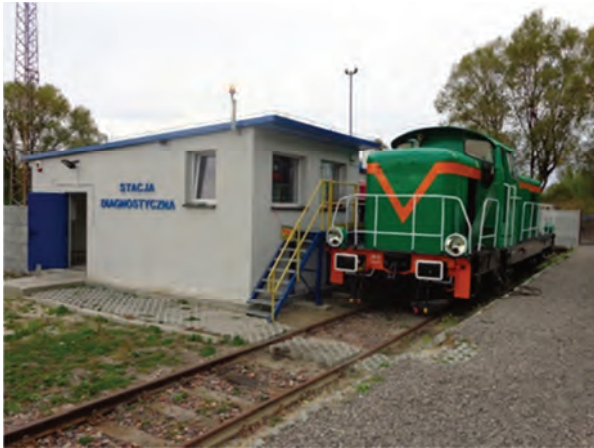
Fig. 4. Diagnostic station for measuring operational parameters and emissions of rail vehicles [20]
