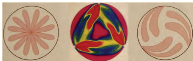
Fig. 11. Shown of the correct injection spray shapes in the injection flow of a four-stroke trunk-piston engine (left), in a large two-stroke crosshead engine with three injectors (centre), and a two-stroke crosshead engine (right) (reproduced from [9])
