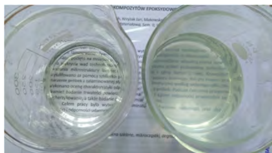
Fig. 2. Comparison optical transparency, a) neat diesel fuel b) nanofuel – Al 2 O 3 50 ppm, turbidity ~30 NTU
