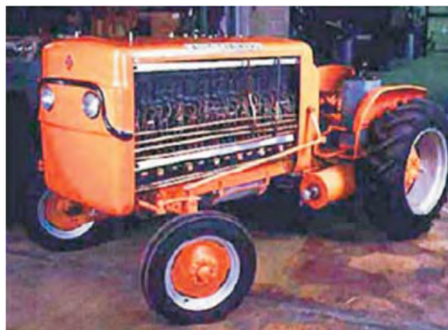
Fig. 21. Allis-Chalmers AC D-12 fuel cell tractor [14, 23]
