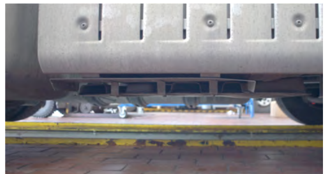
Fig. 3. View of the outlet of the exhaust system – Mercedes Actros truck
