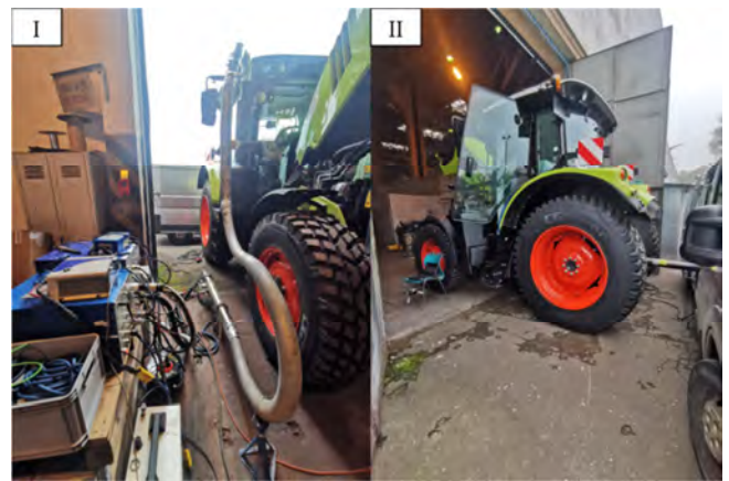
Fig. 2. Test stand: I – exhaust emissions measurement device, II – connection between the PTO and the mobile dynamometer
