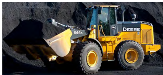
Fig. 11. John Deere 644K Hybrid loader [27]
