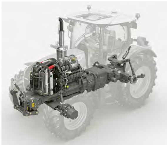
Fig. 1. Test vehicle with the drive system highlighted [10]
