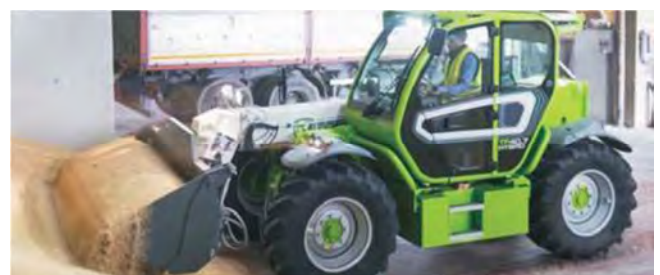
Fig. 36. Merlo 40.7 hybrid telehandler [48]
