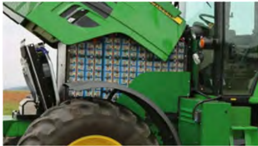
Fig. 23. Battery pack of John Deere SESAM [36]
