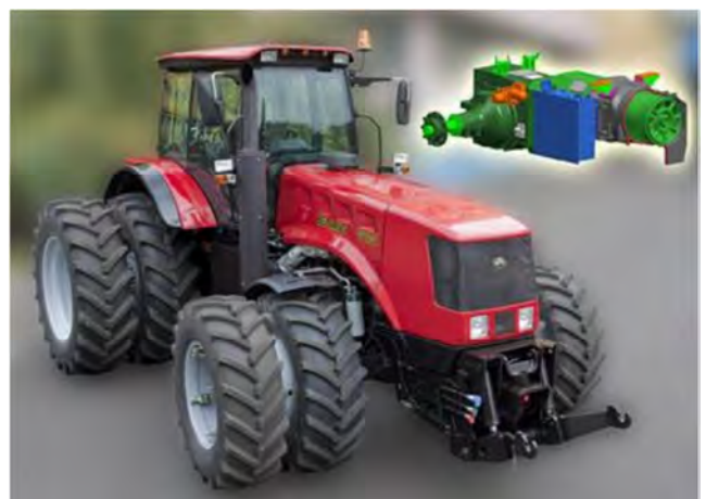
Fig. 7. Belarus 3023 with electro-mechanical powertrain [23]
