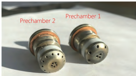
Fig. 5. Used prechambers (jet exit sides)
