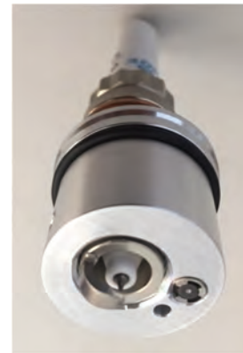
Fig. 14. Assembly of check valve (design 1) into prechamber top lid
