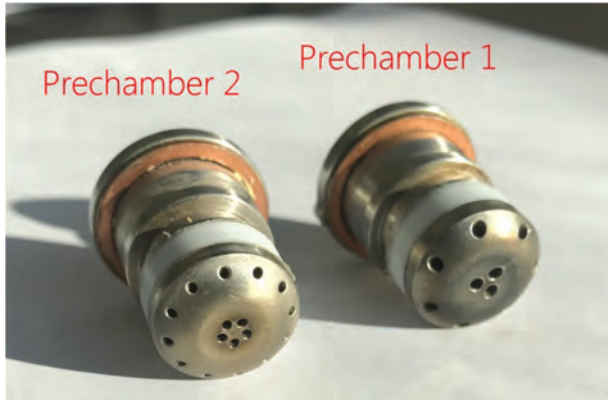
Fig. 7. Two different samples of prechambers with additional nozzles [4]
