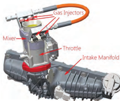
Fig. 2. CAD visualisation of gas mixer, throttle and intake manifold
