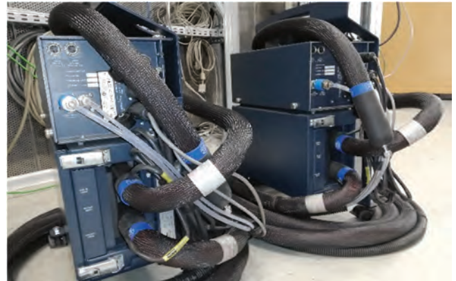
Fig. 13. The prefilters of tailpipe modal measurement of AVL iGEM emission system
