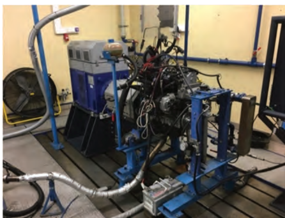
Fig. 5. The test engine mounted on the dynamometer along with the engine control unit
