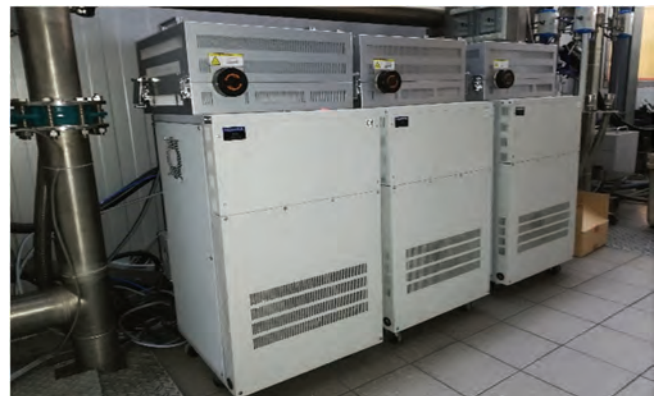
Fig. 14. The Horiba OVN’s of tailpipe modal measurement of Horiba emission system
