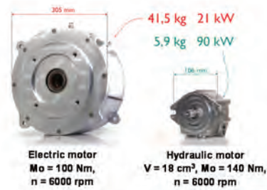
Fig. 8. Technical parameters comparison of electric and hydraulic motors [1]
