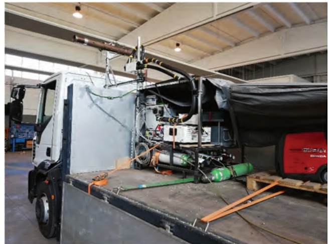
Fig. 2. AVL PEMS system installed on the load carrying area of a heavy duty vehicle
