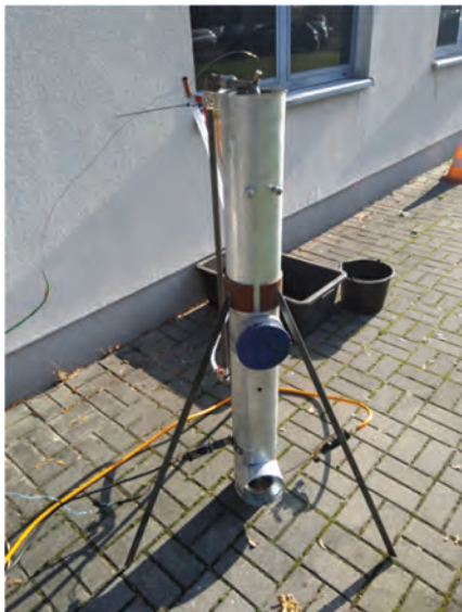
Fig. 7. A reactor for the production of synthesis gas
