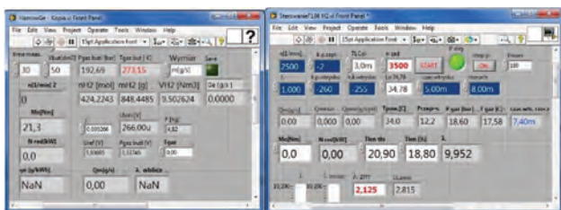
Fig. 5. Windows of the control program controlling the parameters of the eddy current engine brake and the tested engine
