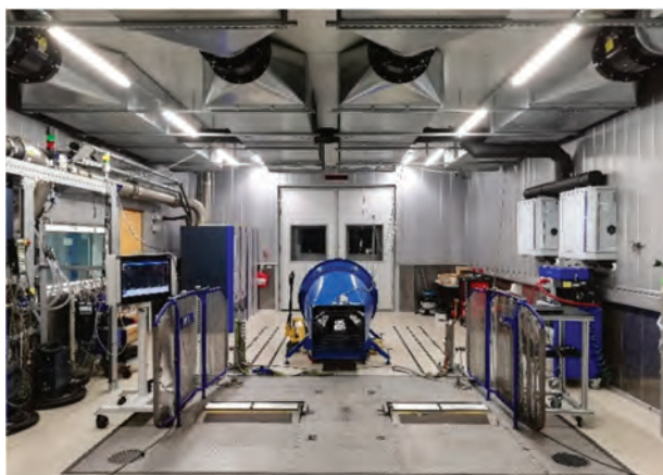
Fig. 2. Internal view of the ambient chamber of Emission Laboratory No. 1, showing the single roller chassis dynamometer and the windspeed fan in front
