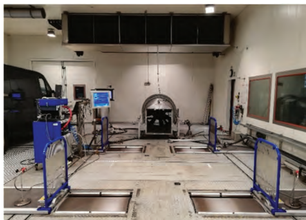
Fig. 4. Internal view of the climatic chamber of Emission Laboratory No. 2, showing the double rollers chassis dynamometer and the windspeed fan in front
