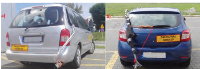
Fig. 2. Cars used for road tests with installed PEMS: a) Euro 3, b) Euro 6
