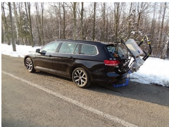
Fig. 1. AVL PEMS system installed on a passenger car. The gas PEMS unit is not visible as it is located inside the vehicle cabin. The PN PEMS, the exhaust flow meter, the sampling line and tubing for re-routing the exhaust are all visible at the rear
