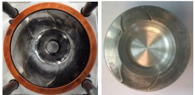
Fig. 2. Piston with a standard (left) and enlarged combustion chamber (right)
