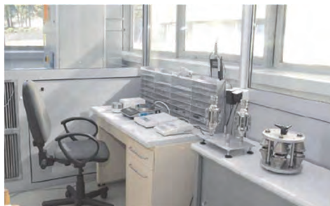
Fig. 11. The balance, filter conditioning racks and filter cartridges in the climate controlled weighing chamber
