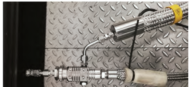
Fig.20. Advance high pressure and temperature option for undiluted emissions measurement of APC AVL device
