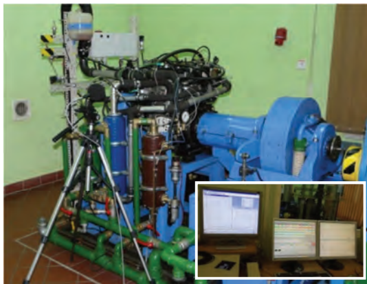
Fig. 6. The engine mounted on the dynamometer stand and the test bench management system monitors [7]
