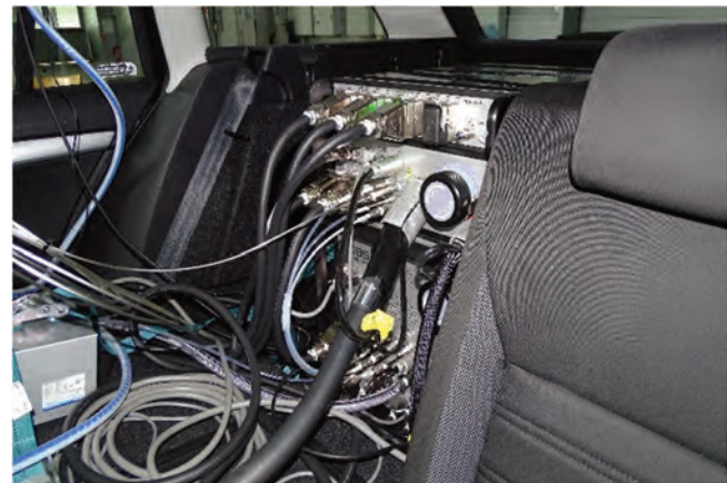
Fig. 24. OBS-ONE HORIBA mounted inside a passenger car for an RDE test
