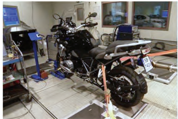
Fig. 6. View of a motorcycle positioned on the chassis dynamometer in Emission Laboratory No. 2
