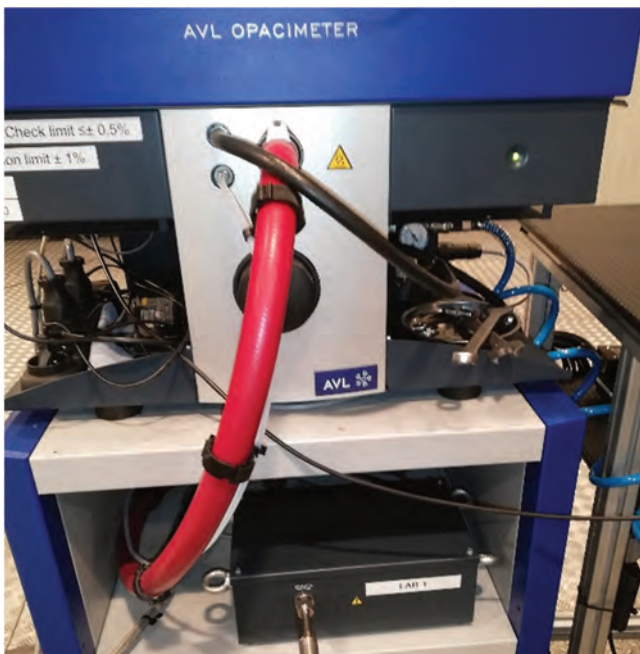
Fig. 18. AVL439 Opacimeter with high pressure optional unit (below)
