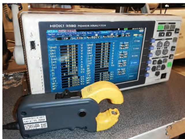
Fig. 12. Hioki Power Analyzer PW3390 with the current probe using as a set (Horiba system) or as a standalone device (AVL iGEM system)
