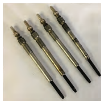
Fig. 3. Standard glow plugs (heating section length – 30 mm)
