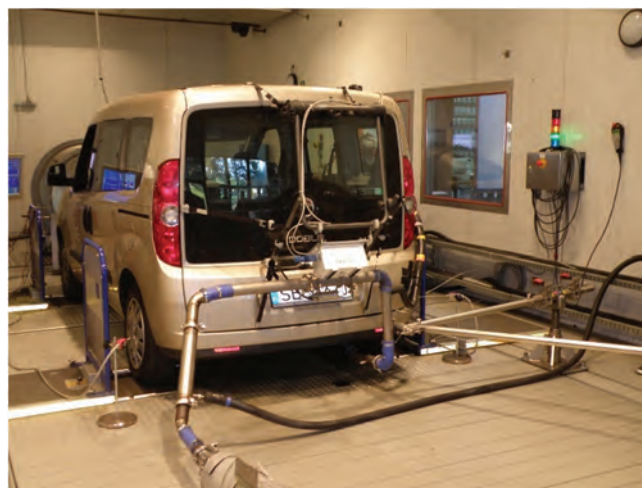
Fig. 5. PEMS system installed on a light duty vehicle undergoing an RDE simulation test on the chassis dyno.
