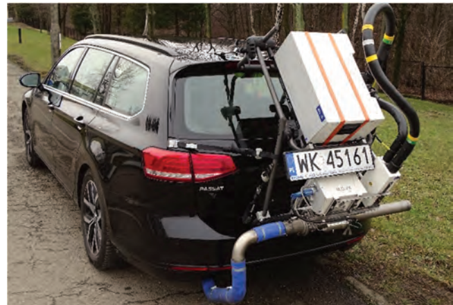
Fig. 23. M.O.V.E. GAS PEMS and M.O.V.E. PN PEMS mounted on a passenger car for an RDE test
