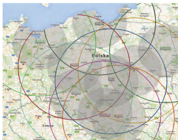
Fig. 5. Penetration area of cars using fuel cells based on 9 hydrogen refuelling stations situated on the national TEN-T road network by the 2030 [3] a) when driving in one direction (diameter of large circles – to approx. 600 km), b) when driving there and back (diameter of small, shaded circles – to approx. 300 km) [17]
