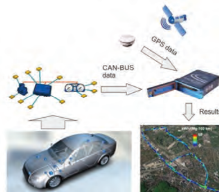
Fig. 1. System used for measurement of car and engine operating parameters
