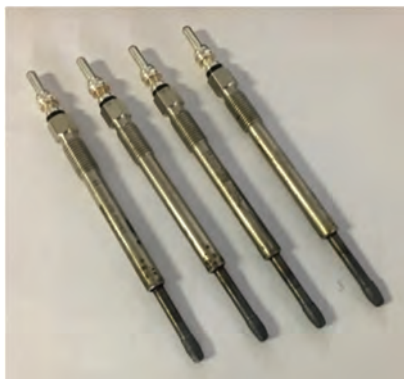
Fig. 4. Prototype glow plugs with an extended heating section length (34 mm)
