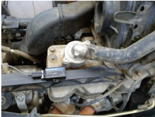
Fig. 2. Placement of the 3DM-GX3-25 sensor on the vehicle during tests
