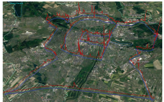
Fig. 5. Local ambient PM concentration during road tests [10]
