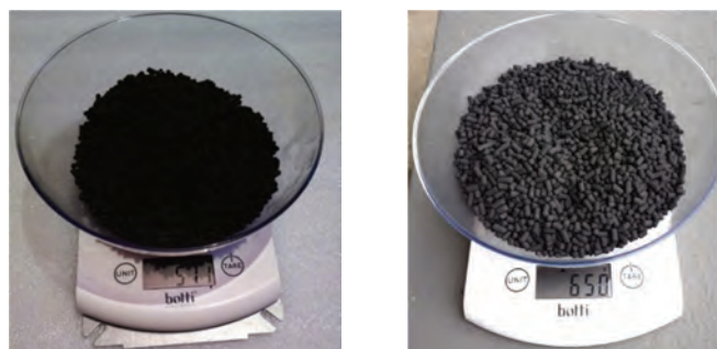
Fig. 8. Weighting of 1 l of activated carbon. Left side – clean carbon – 511 g, right side carbon after 4 months of operation – 650 g
