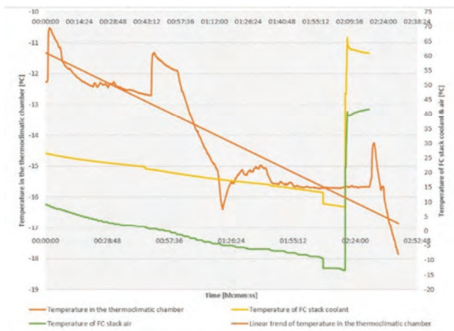
Fig. 3. The temperature of the cooling medium of the fuel cell stack and the air in the cell segments, during the tests of the vehicle in the thermoclimatic chamber
