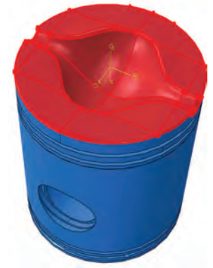
Fig. 7. The boundary condition of the piston thermal load – bottom – temperature: 850 K, heat transfer coefficient: map
