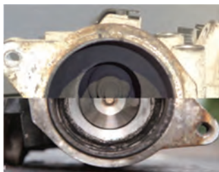
Fig. 3. Comparison of two pictures of EGR valve channels: channel with sediments (top picture), channel after partial removal of sediments with chemicals (bottom picture)
