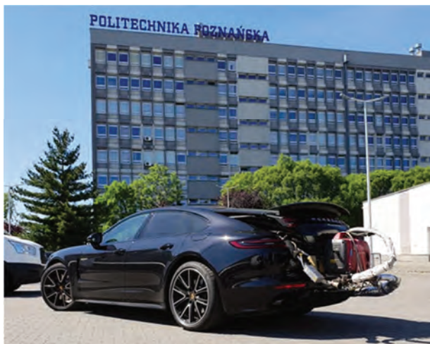
Fig. 1. The tested vehicle with PEMS apparatus
