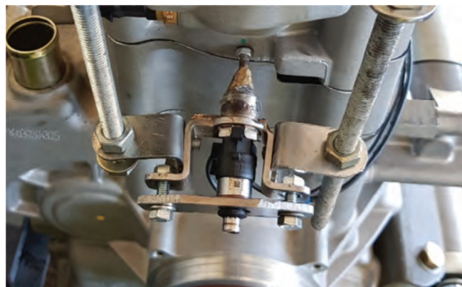
Fig. 9. Cylinder head with extraction channel and installed valve
