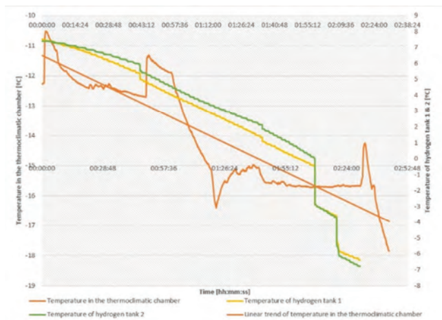
Fig. 6. Temperature of hydrogen tanks during vehicle tests in a thermoclimatic chamber
