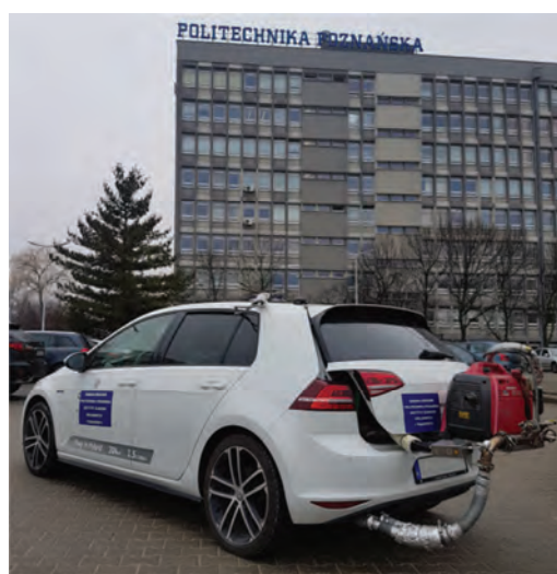
Fig. 3. The test vehicle equipped with the PEMS device during tests in real operating conditions
