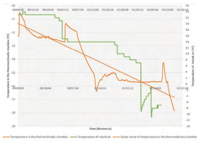
Fig. 4. Air temperature in the fuel cell intake system during vehicle tests in the thermoclimatic chamber
