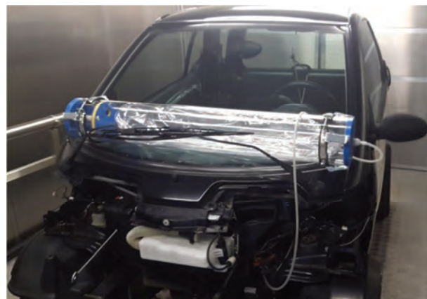
Fig. 5. Exterior of the tested vehicle with sampling probe
