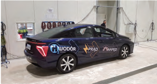
Fig. 1. Toyota Mirai during tests in the thermoclimatic chamber
