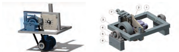
Fig. 4. Torque measuring system on the high-pressure pump shaft: 1 – high pressure pump, 2 – mounting plate, 3 – frame, 4 – frame pins, 5 – bearing housing, 6 – distance column, 7 – load cells sensor
