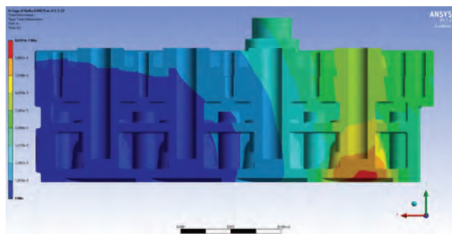
Fig. 15. Distribution of total deformations as result of simulation of the first cylinder loading – longitudinal section
