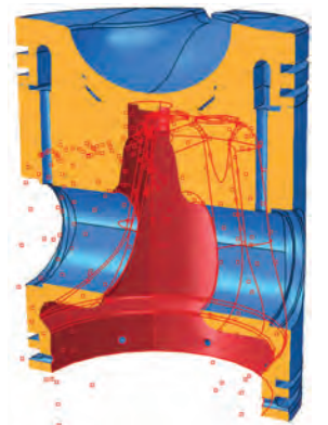
Fig. 9. Additional boundary condition for the thermal load of the piston – internal surfaces – temperature: 393 K, heat transfer coefficient: 500 W/(m 2 K)
