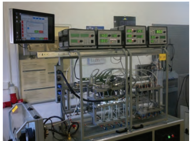
Fig. 4. Diesel Bench STPiW-3 main diagnostic test bench
