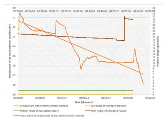
Fig. 7. Hydrogen pressure in high, medium and low pressure circuits during vehicle tests in a thermoclimatic chamber
