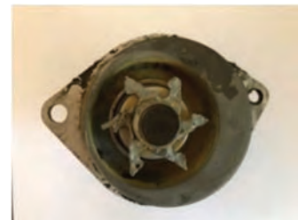
Fig. 2. A mechanical coolant pump destroyed by the erosive action of cavitation
