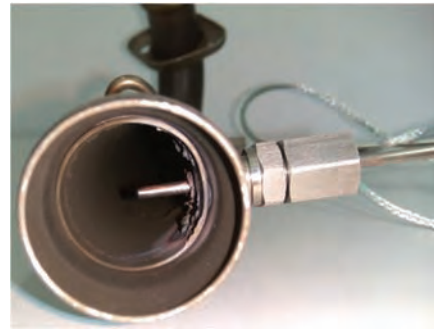
Fig. 4. Temperature sensor mounting
