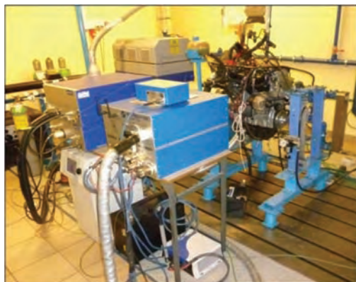
Fig. 3. Dynamometer test bench with the measuring apparatus
