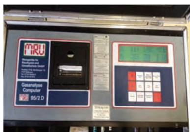
Fig. 2. Exhaust gases analyzer type MRU 95/3CD
