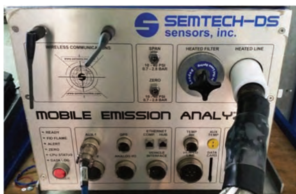
Fig. 3. The SEMTECH DS mobile analyzer used in the Ford Focus Flexifuel vehicle tests
