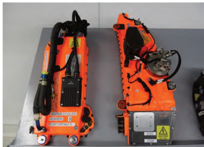
Fig. 6. First track test KERS battery and power electronics from 2008
