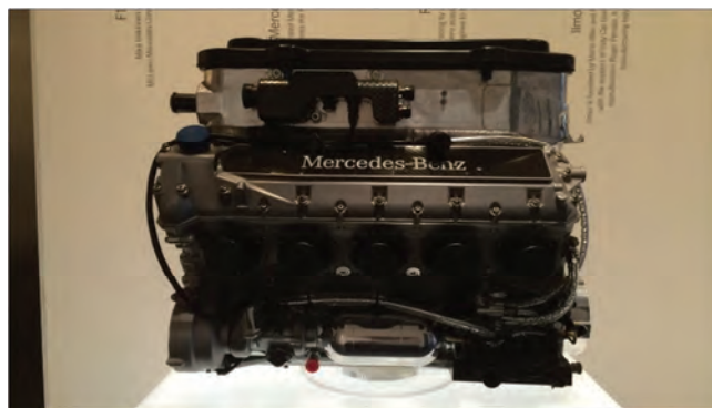
Fig. 4. Mercedes-Benz Fo 110, 3000 cm 3 , V10 engine for 1995 F1 season
