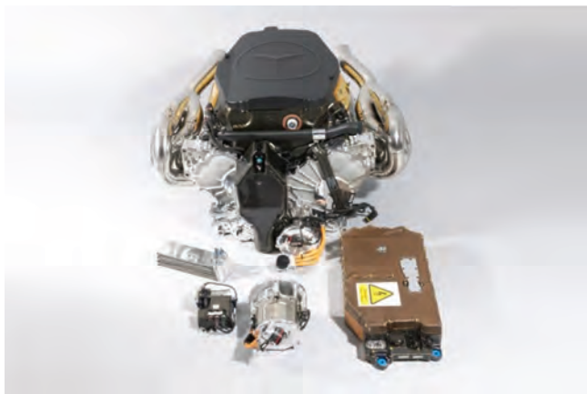
Fig. 7. Mercedes-Benz FO 108 W, 2400 cm 3 , V8 with KERS for 2009 F1 season [25]
