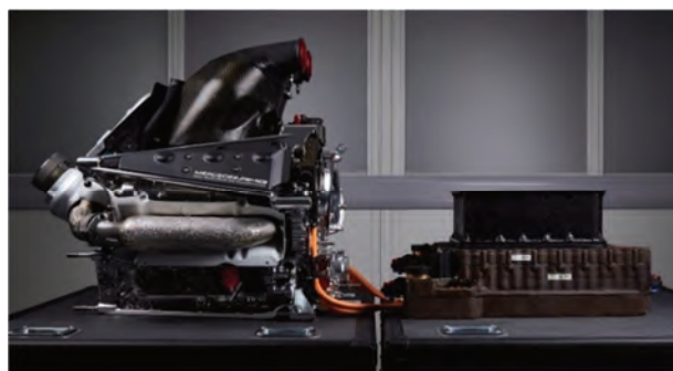
Fig. 9. Mercedes-Benz PU 106 A Hybrid, 1600 cm 3 , V6 power unit for 2014 F1 season [25]
