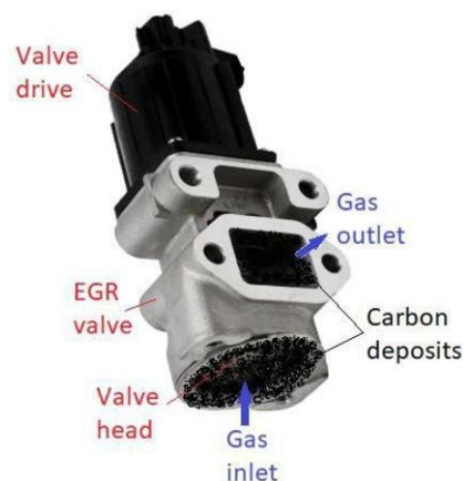
Fig. 1. EGR-valve covered with Carbon Deposits (CDs)
