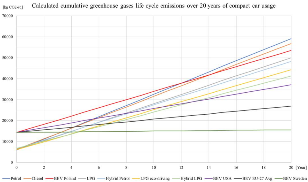
Fig. 2. Calculated cumulative greenhouse gases life cycle emissions over 20 years of compact car usage
