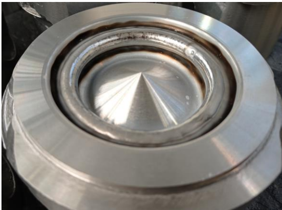
Fig. 8. Combustion chamber of an aluminum piston after the local DuralBowl remelting process
