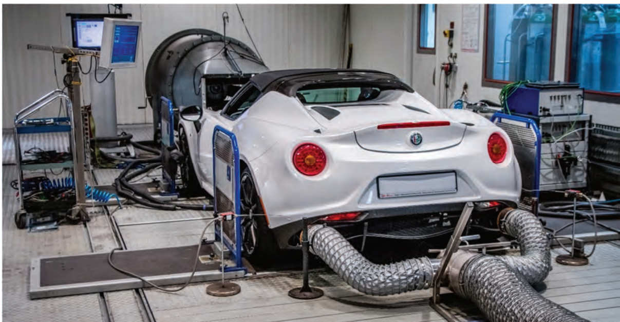
Fig. 13. BOSMAL's climate-controlled 4WD chassis dynamometer for R&D and certification work on conventional, hybrid and fully electric powertrains
