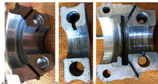
Fig. 20. Appearance of worn bearing bushings of cam roller bearings on the side of bearing covers, a) bearing 3, b) bearing 2, c) bearing 1
