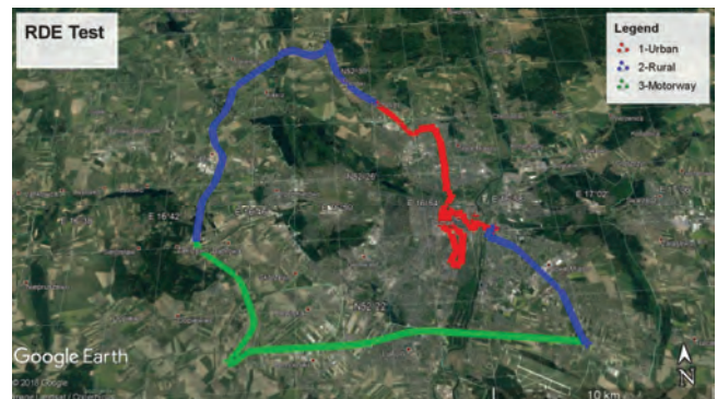
Fig. 2. The research route with marked RDE test phases
