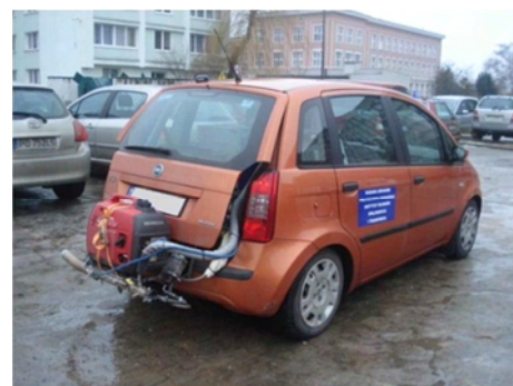
Fig. 1. Fiat Idea with mounted exhaust measuring apparatus [1]
