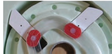
Fig. 4. a) Prototype of the vane engine by K. Rządkosz, b) mechanism for guiding baffles in the engine
