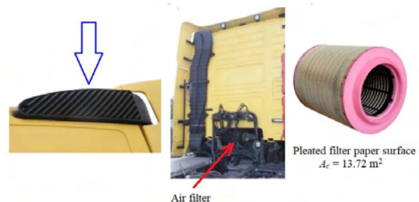
Fig. 4. Air supply system for the engine of a Volvo FH13 truck tractor: a) air intake, b) general view of the air supply system, c) paper filter cartridge
