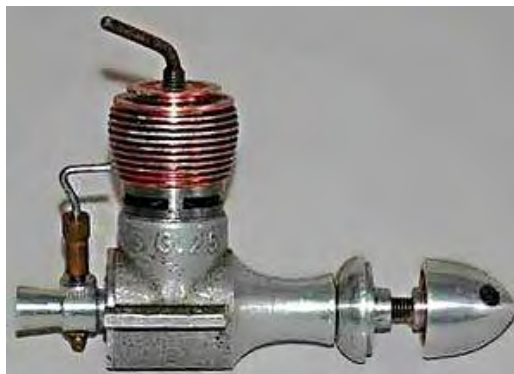
Fig. 3. Polish self-ignition engine “Jaskółka” with a capacity of 2.5 \text{ cm}^3 [26]
