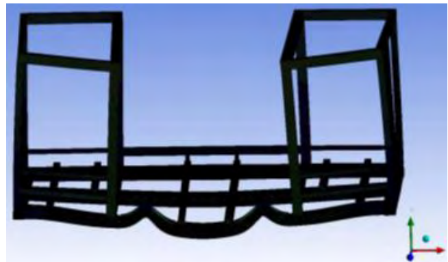
Fig. 6. Visualization of the mechanical load model of the mobile dynamometer structure
