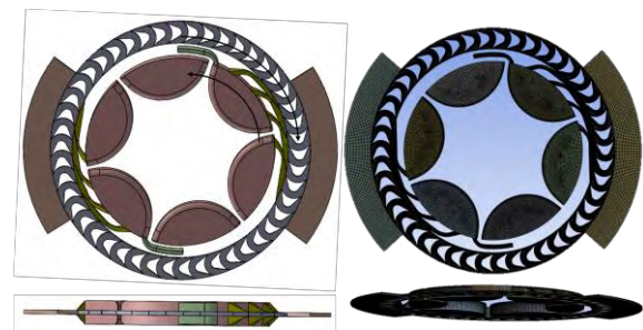
Fig. 1. Geometry model and numerical mesh—engine concept of 500 kW power
