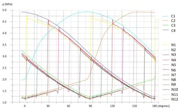
Fig. 12. Pressure change of the gas in chambers (C1, C2, C3, C4) and nozzles (N1-N12) for 180 degrees rotation of chambers (2 engine cycles)
