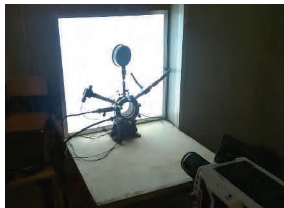
Fig. 1. Test bench with isochoric combustion chamber
