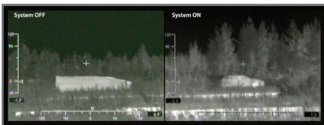
Fig. 7. Thermal masking method ADAPTIV from BAE Systems [8]
