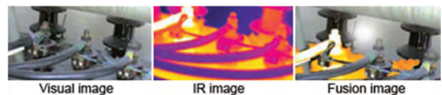
Fig. 2. Comparing images (from left side) in visible light, in infrared and using fusion technology [1]
