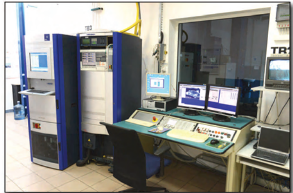
Fig. 2. A set of analysers AMA i60 R2 and CEB II
