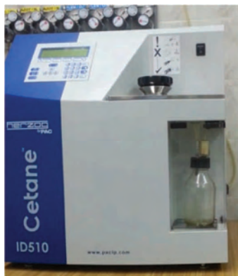
Fig. 1. Device for determination of derived cetane number CID 510
