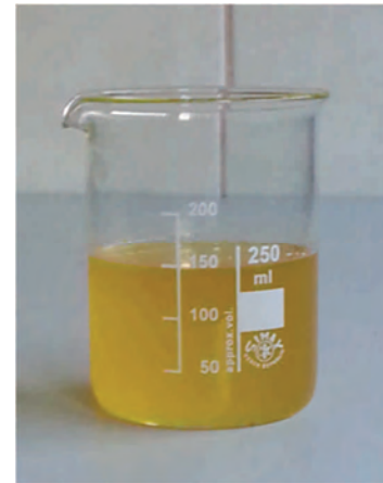
Fig. 2. Diesel fuel blend with 15% volumetric content of ethanol
