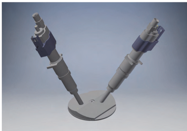
Fig. 4. The indicative view of positioning the direct injection fuel injectors
