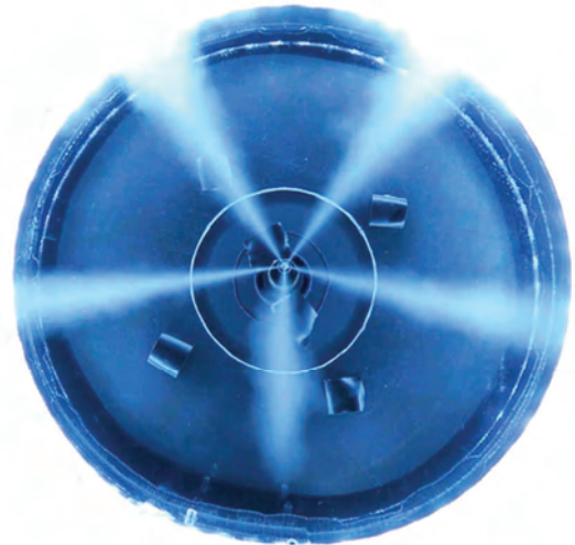
Fig. 20. Fuel spray pattern of a damaged injector
