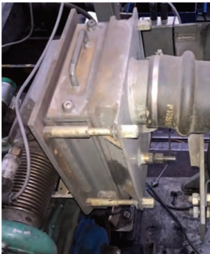
Fig. 2. Flame arrester used in a mine combustion engine
