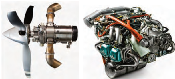
Fig. 11. Aircraft turboshaft TP-100 engine (right) [15] and Rotax 912-ULS spark ignition engine (left) [13]
