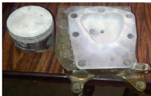
Fig. 1. The elements of engine covered by means of plasma spraying
