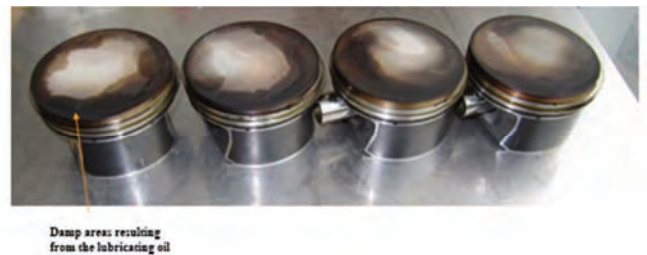
Fig. 8. State of the catalytic surface after 28 hours of operation
