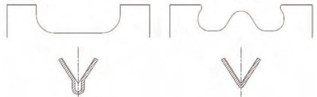
Fig. 11. Geometry of the combustion chamber and the nozzle endings; standard version – left, modified version – right [11]
