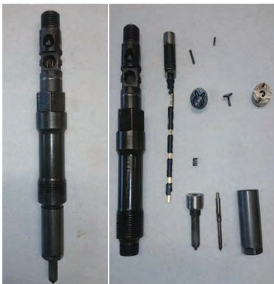
Fig. 8. A – electromagnetic Delphi fuel injectors, B – electromagnetic Delphi fuel injector disassembly on spare parts
