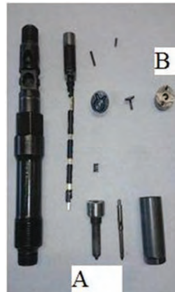
Fig. 5. Electromagnetic Delphi fuel injector dismantled on spare parts: A – injector nozzle area, B – steering valve and electromagnetic coil area
