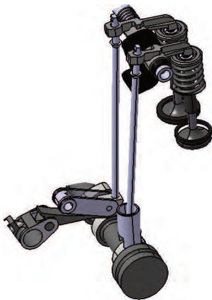
Fig. 1. The scheme of valve train from the engine for tribological studies
