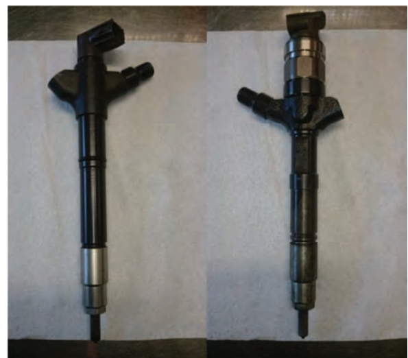
Fig. 6. Denso fuel injectors A – piezoelectric, B – electromagnetic
