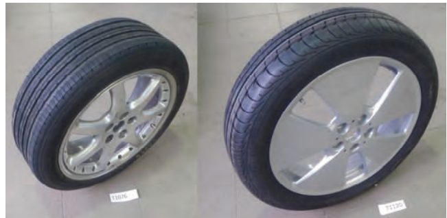
Fig. 7. Tyres for electric cars; on the left – tyre of typical size for modern cars with conventional design, on the right – tyre for electric cars constructed in nonorthodox way
