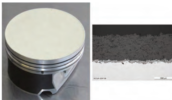
Fig. 7. Piston surface coated with zirconium oxide
