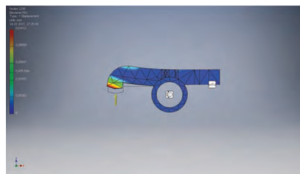
Fig. 20. The displacements of points of the rocker arm sub-model loaded by the force F=1000 N on the valve side
