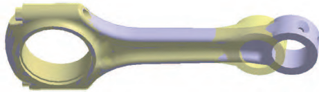
Fig. 15. Geometric changes between model 5 (gray) and model 6 (yellow)
