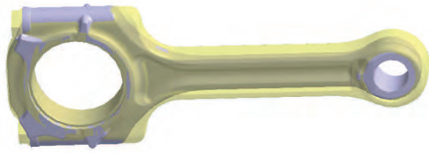
Fig. 7. Geometric changes between model 1 (gray) and model 2 (yellow)
