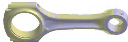
Fig. 19. Geometric changes between model 7 (yellow) and model 8 (gray)
