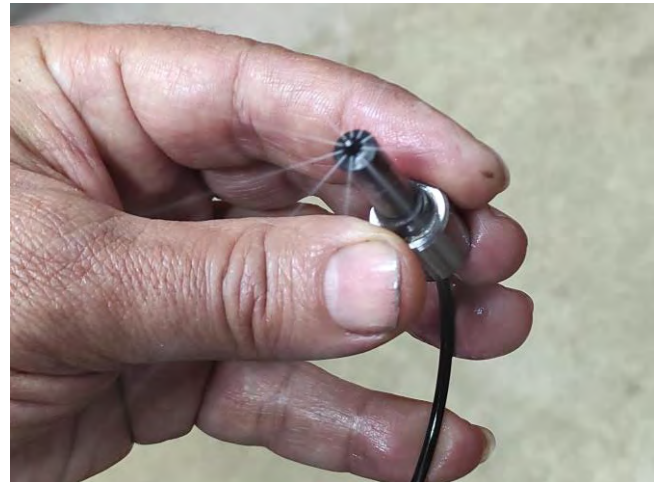
Fig. 6. Checking the patency of the nozzle openings
