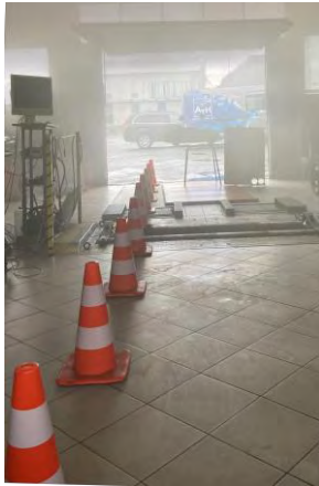
Fig. 3. Test stand for measuring the effects of fog on lidar performance
