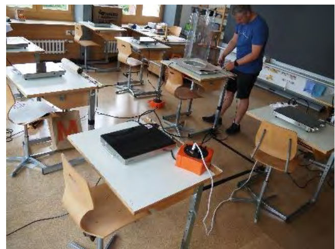
Fig. 21. Researcher installs the particle source at one desk, all other desks have particle counters and heated plates to simulate the students
