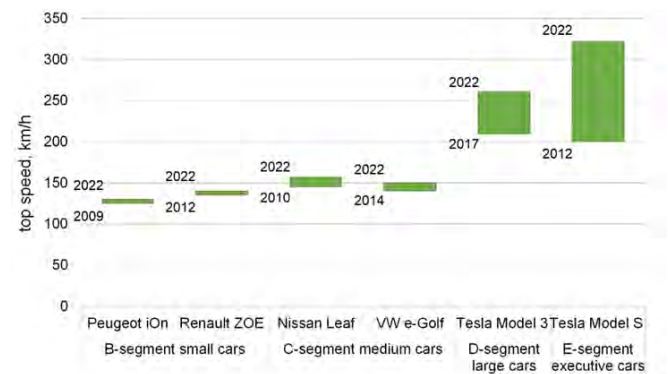
Fig. 2. The top speed of the selected electric vehicle models analyzed from the start of their production until 2022
