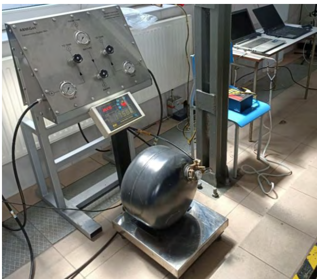
Fig. 2. Stand for preparing of LPG/DME blends
