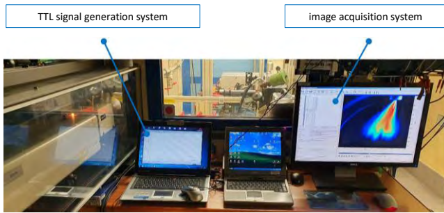
Fig. 4. View of the control panel for the operation of a test stand equipped with an isochoric chamber
