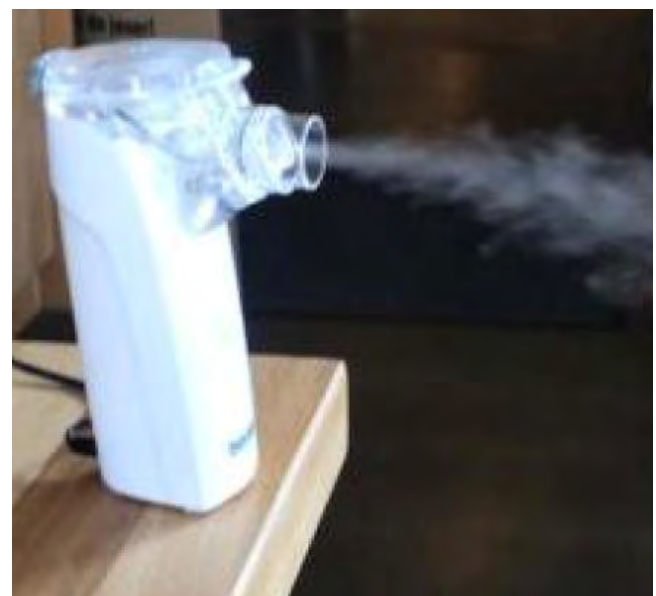
Fig. 22. Nebulizer is used to form a spray of salt solution droplets, drying fast, forming a cloud of 30 nm particles, about 80'000 per cc
