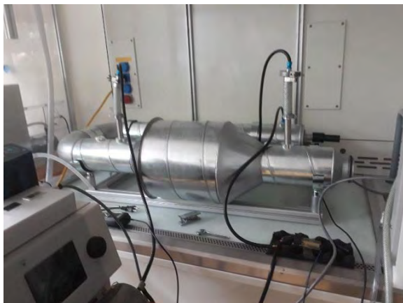
Fig. 6. Actual test installation at FHNW with aerosol sampling points for particle counting
