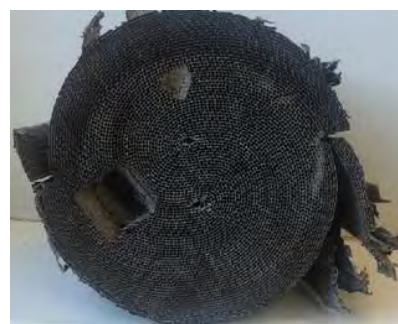
Fig. 4. Catalytic reactor metal support used for X-ray analysis and recycling [6]
