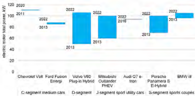
Fig. 7. Electric motor total power of the selected PHEV models from the start of their production until 2022
