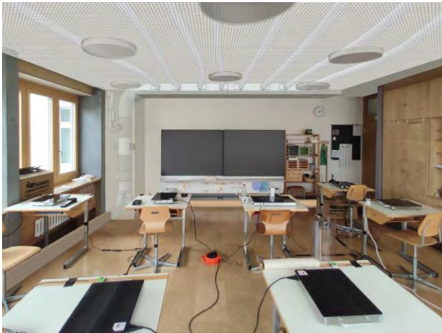
Fig. 14. Pilot classroom with hot plates to replace the students body heat
