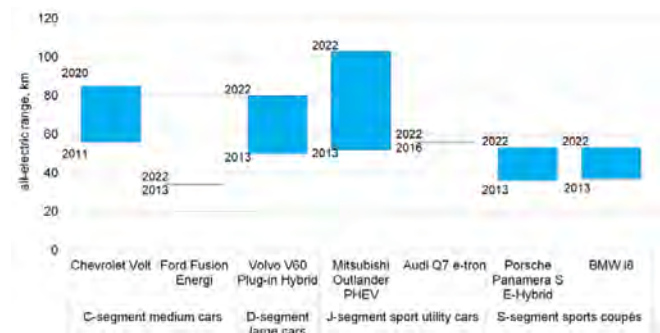
Fig. 9. The electric range of the selected PHEV models from the start of their production until 2022
