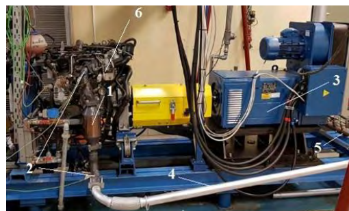
Fig. 9. Test stand: 1 – particulate filter, 2 – temperature measuring points, 3 – electric motor of dynamic dynamometer, 4 – exhaust system, 5 – exhaust gas flow meter, 6 – internal combustion engine
