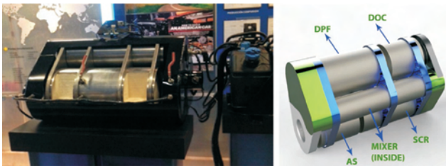
Fig. 3. Concept of Close Coupled SCR system in HD application
