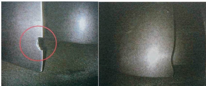
Fig. 5. Comparison of the fan vanes of the RD-33 engine before and after polishing
