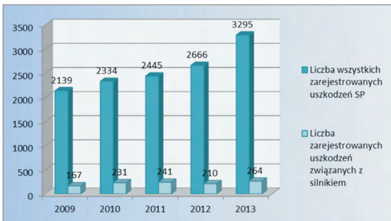
Fig. 1. Number of aircraft incidents related to the malfunctioning powertrain in the Polish Air force in the years 2009-2013
