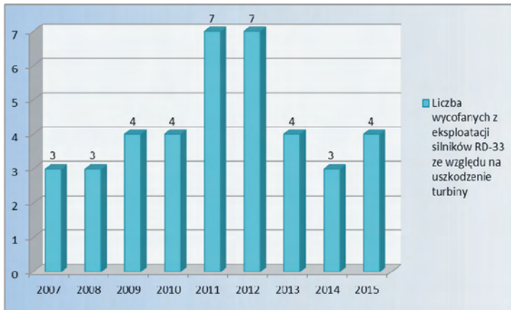
Fig. 6. The number of RD-33 engines withdrawn from operation due to the damage of the high-pressure turbine in the 23 BLT in the years 2007-2015
