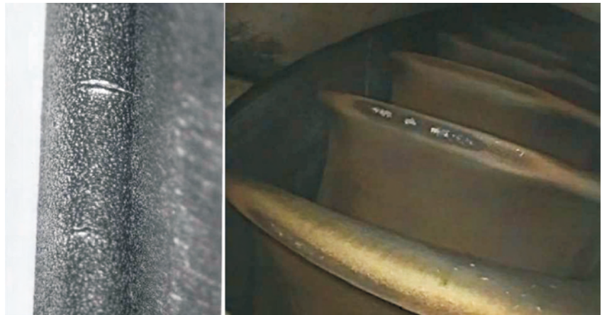
Fig. 7. Examples of damage to the high-pressure turbine vanes of the RD-33 engine
