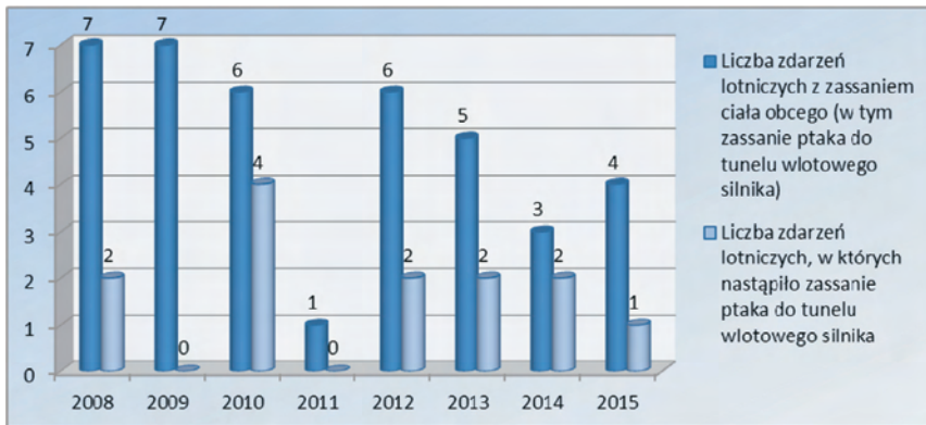
Fig. 4. Number of incidents of RD-33 engine damage related to the ingress of a foreign object in the Polish Air Force in the years 2008-2015
