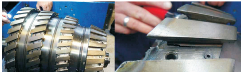
Fig. 8. Example of a fatigue crack of the discs of the IV stage of the RD-33 engine fan (on the left – view of the entire rotor, on the right – visible crack)
