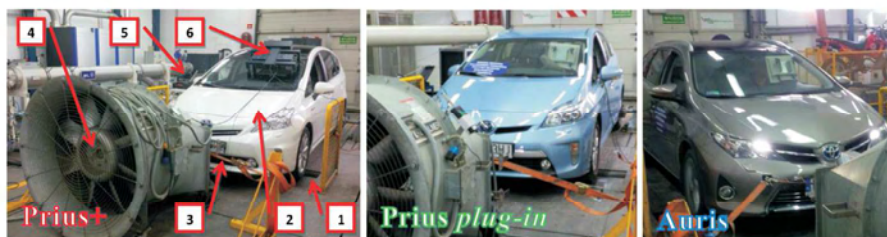
Fig. 6. Test stand: 1 – chassis dynamometer, 2 – tested vehicle, 3 – protection belts, 4 – fan, 5 – diagnostic computer, 6 – monitor showing the UDC drive test parameters
