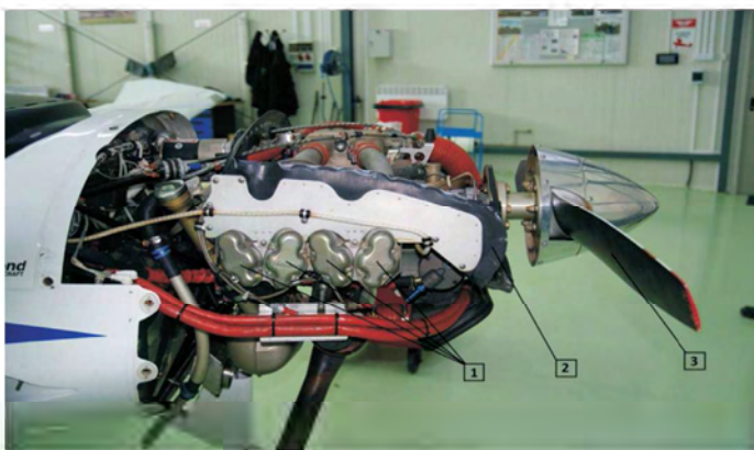
Fig. 4. The propulsion system of the Diamond DA20-C1 "Katana" aircraft: 1 – the valve cover, 2 – baffles, 3 – propeller
