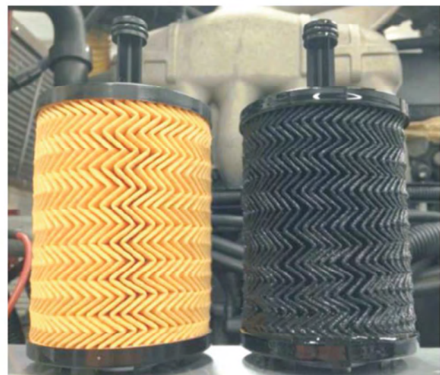
Fig. 8. New oil filter (left) and a filter removed after two minutes operation in the engine oil which contained a residue of carbon nanotubes (right)
