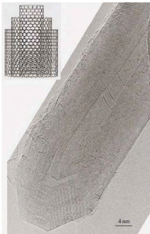
Fig. 3. Multi-walled carbon nanotube with a concentric spatial structure (c-MWNT); image obtained with TEM microscopy [5]
