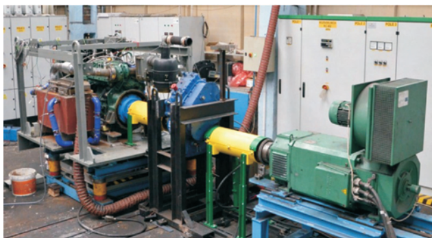
Fig. 7. General view of test stand for diesel drive [7]
