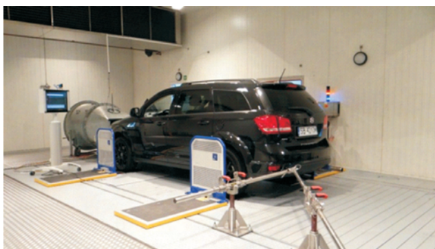
Fig. 3. Modern Emission Laboratory with 4WD chassis dynamo
