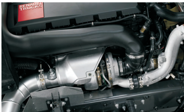
Fig. 7. The seventh injector in the exhaust manifold and the flap valve downstream of the turbine [9]
