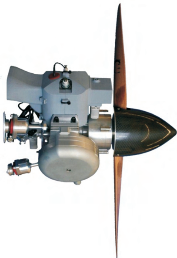
Fig. 21. NW-44 EFI HFE engine; basic configuration [27]
