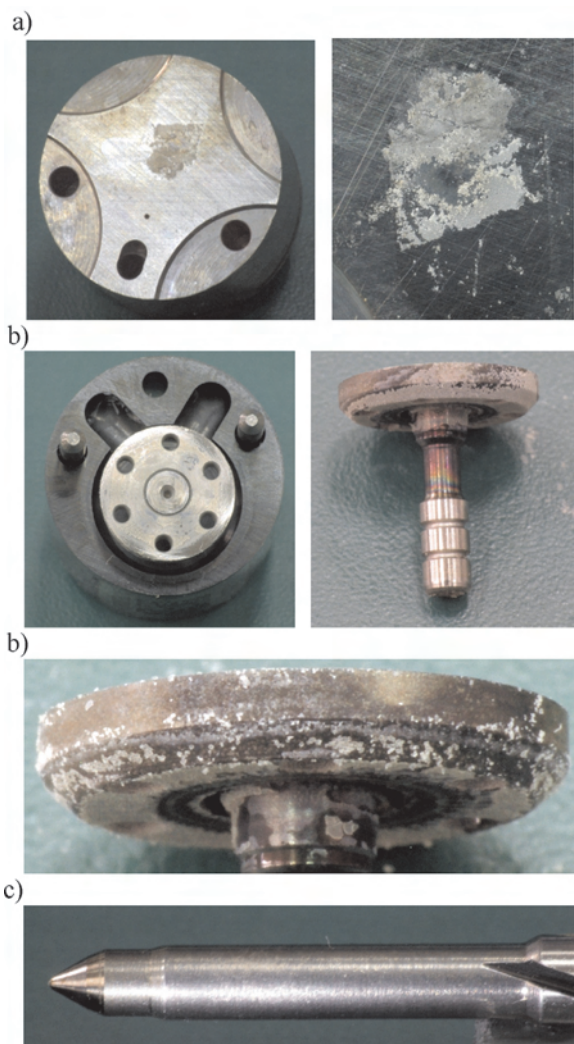
Fig. 3. Deposits (type I) on internal elements of injectors of HPCR system: a) body of chamber controlling fuel flow, b) body of control valve and control piston of electromagnetic valve, c) nozzle needle
