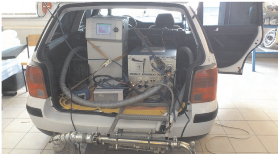
Fig. 3. PEMS measuring equipment during installation inside the vehicle
